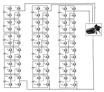
Fig. 6: Structure of thirteen level Inverter
