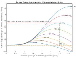
Fig. 15: Wind Generator power curves at various wind speeds
