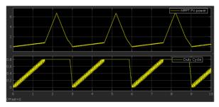
Fig. 13: Simulation output of power and duty cycle from a MPPT Controller
