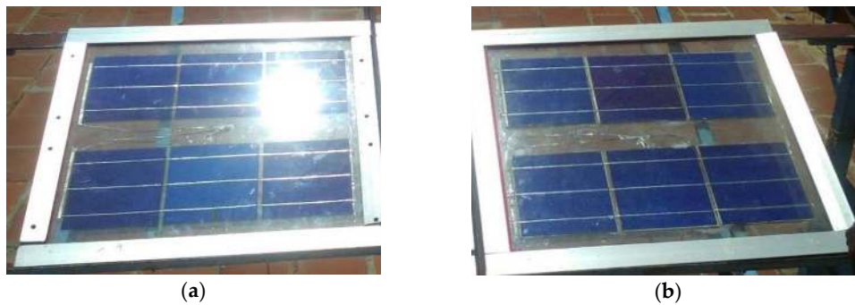
Figure 3. Photographic view: (a) STPV module without PCM; (b) STPV module with PCM.
