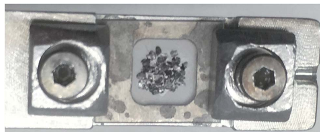
Fig. 2 A photograph of the mosaic of CrSe 2 single crystals affixed to a sapphire plate (Crystal GmbH, Berlin) using Apiezon-L grease (M & I Materials, Manchester). The tight packing and highly focused 8 Li + beam spot used in the experiment minimizes the β-NMR signal from the surrounding materials.
