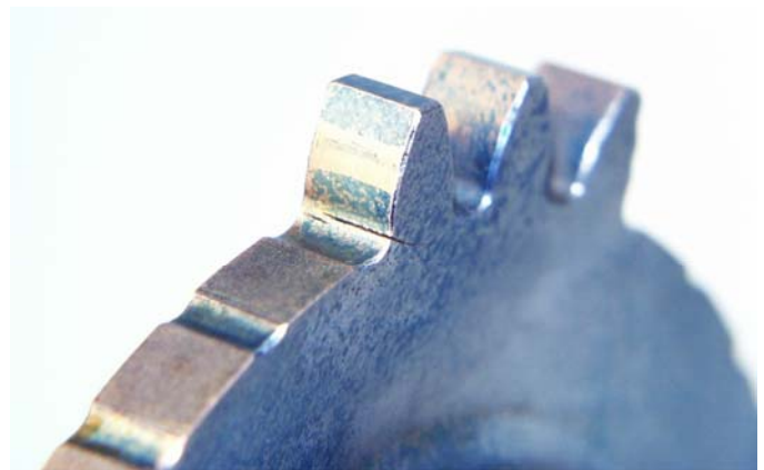
Figure 6.—Single tooth bending failure at test termination.
