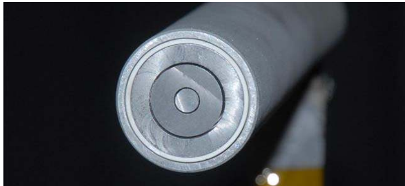
Figure 3-25 Photograph of the AFRL nested Faraday probe shown in the 0.5 mm gap width configuration.
