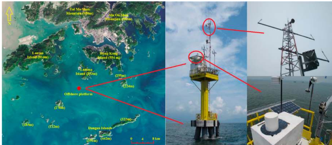
Figure 1. Location of measurement site (highlighted in solid red circle) and wind measurement system (upper: met mast; bottom: wind Lidar).
