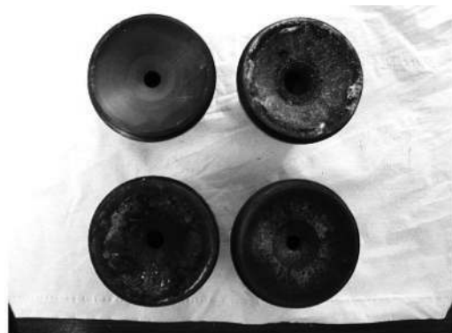
Fig. 4 Clockwise from top left: new, Al/HTPB test, Al-Mg/HTPB test, and HTPB test.
