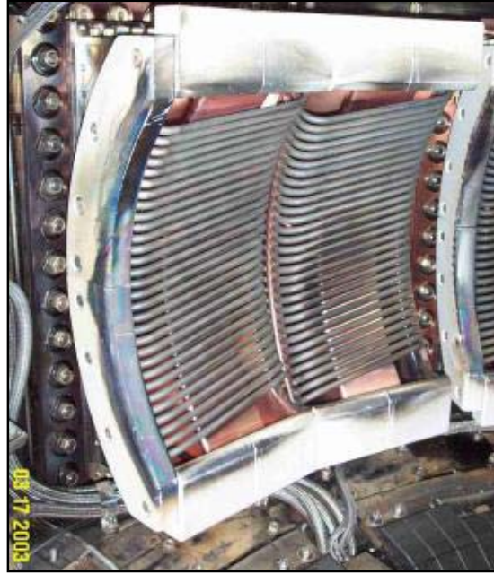
Figure 1: D antenna with BN (white) tiles installed.
