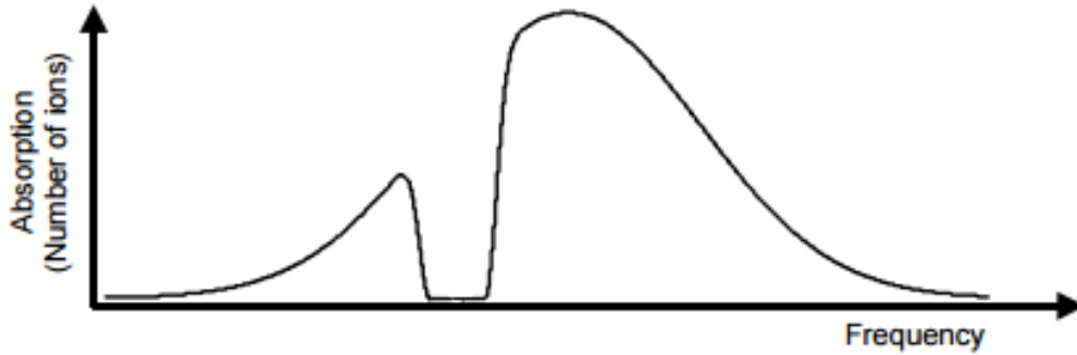
Figure 3.3: Inhomogeneous broadening of absorption profile with a spectral pit (not drawn to scale). Figure adopted from [39]
