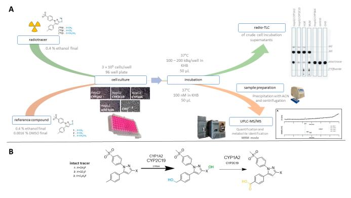
**Figure 1.** Established workflow for investigating the metabolism of radiotracers. (**A**) Workflow for incubations with radiotracers (green arrow) and for nonradioactive reference compounds (orange arrow). (**B**) Sites for oxidative metabolism in [<sup>18</sup>F]1–3 [28,29].
