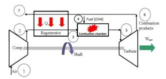
Figure 2. Regenerative gas turbine power plant
