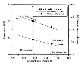
**Figure 1.** Effect of entry temperature on the power output and power generation efficiency of the GT [2]
