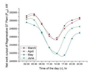
**Figure 5.** Network output of regenerative GT plant Vs. time of the day (peak temperature day of the month)
