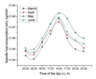
Figure 8. Specific fuel consumption Vs. time of the day (peak temperature day of the month)
