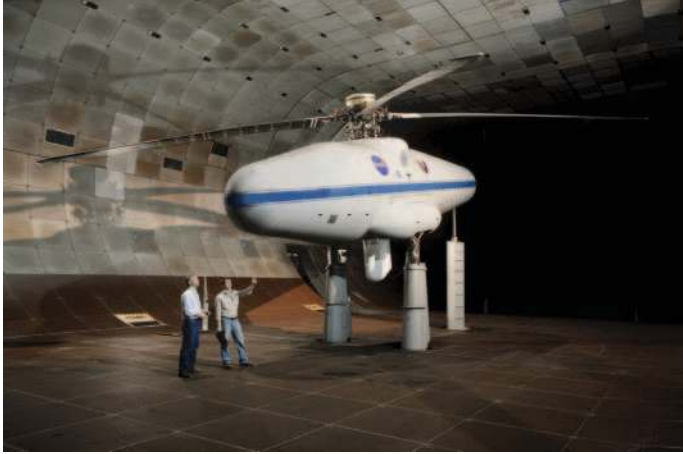
Fig. 1. UH-60A rotor system installed on the LRTA in the NFAC 40-by 80-Foot Wind Tunnel.
