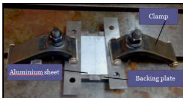
Figure 2. Clamping in CNC milling machine.
