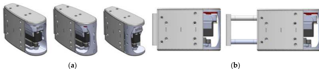
Figure 8. Snake robot modules a) Revolute motion of module b) Linear motion of module.
