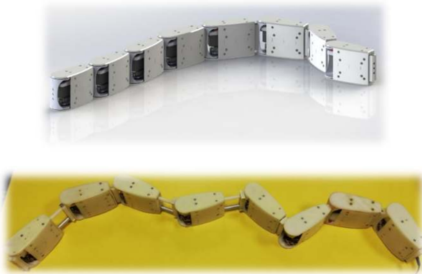
Figure 11. CAD model (top) and experimental snake robot (bottom).
