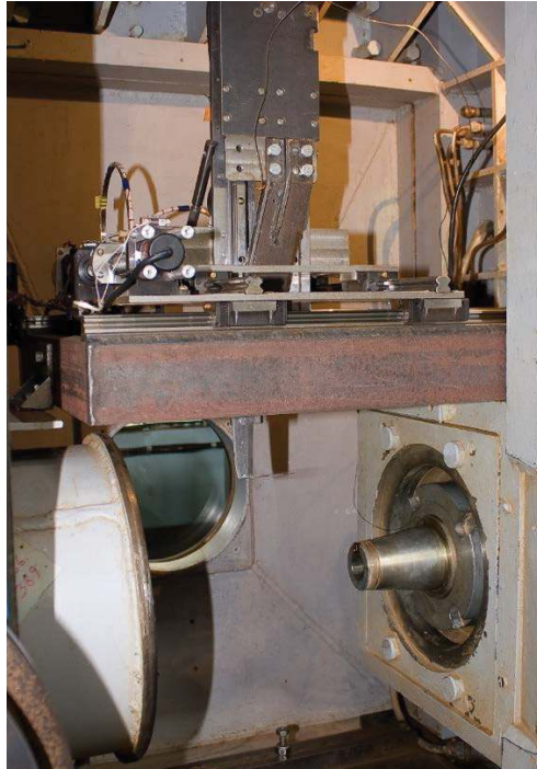
FIGURE 1.1 Photo of the test chamber of the jet module of the wind tunnel T-326 ITAM SB RAS
