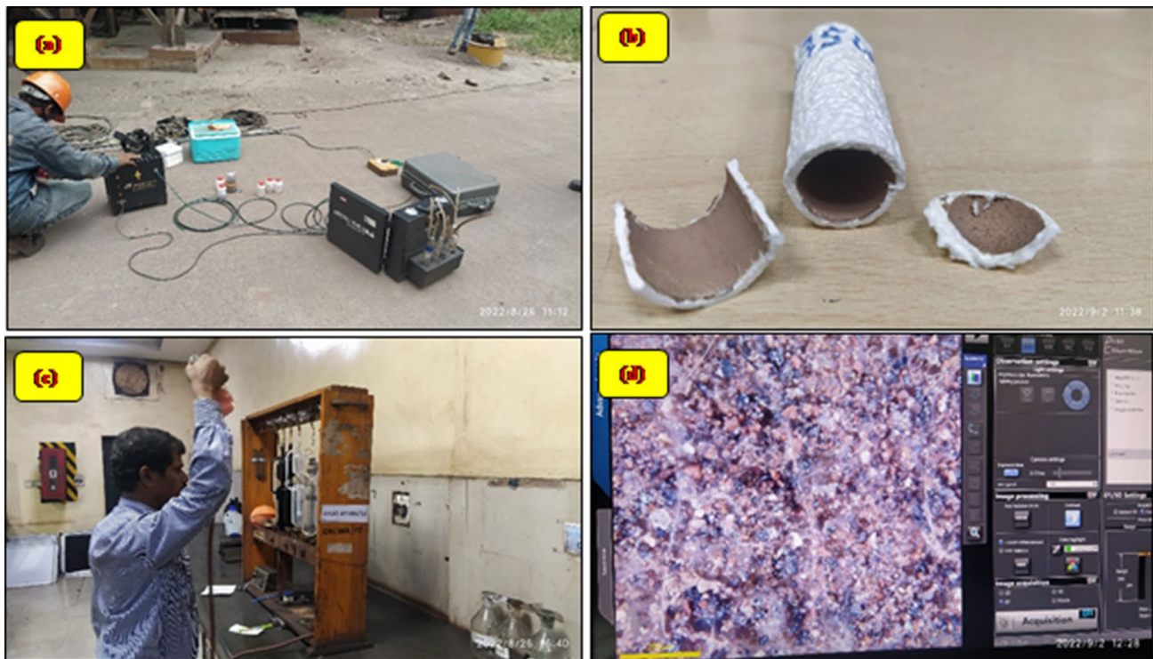
Fig. 4 a Stack sampler kit, b the deposit of particulates in a thimble, c Orsat apparatus, d optical micrograph
