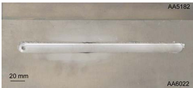
Fig. 5 Friction stir lap welded AA 6022-5152 sheet
