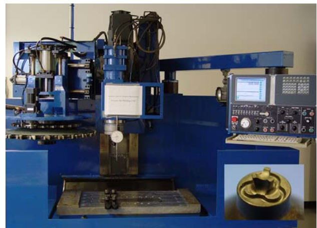
Fig. 1 CNC-controlled friction stir welding with 2D welding capability. Inset: Tool used for friction stir lap welding of aluminum sheets
