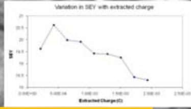
Clockwise from bottom left: 1) SEM micrograph of a CVD diamond surface showing "ageing", dark regions are previously imaged areas. 2) Before (top) and after (bottom) photos of the Faraday cup on the target arm after prolonged E-beam illumination showing EBD. 3) A plot showing SEY versus E-beam energy for a number of tested samples. 4) Typical degradation in the SEY with extracted charge. 5) Variation of SEY with E-beam angle of incidence (an unexpected result awaiting investigation)
