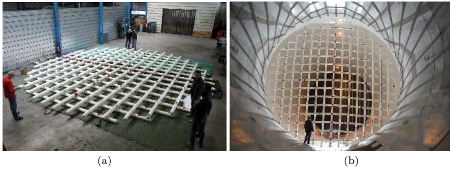
Fig. 2 (a) First assembly of the grid. (b) Final assembly of the grid in the convergent section of S1MA windtunnel.
