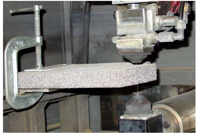
Fig. 1. Setup of the wire EDM machining of a metal foam plate.
