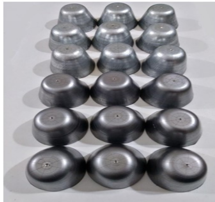
Figure 6: Photographs show the cups produced from different die wall angles, punch velocities, material types, and sheet thicknesses.
