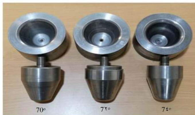
Figure 5: Photograph shows the punches and dies used in this study.
