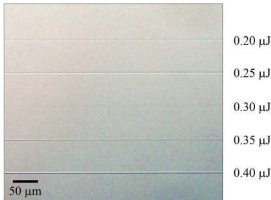
Fig. 9. Linear structures written with a translation speed of 25 \mu\text{m/s} in phosphate glass using the 50\times ( 0.8 \text{ NA} ) microscope objective and various pulse energies measured after a 900 \mu\text{m} slit. The top two structures guide light indicating a positive index change. The bottom two structures do not guide light representing a negative index change. The structure in the middle shows the transition between a positive and negative index change.
