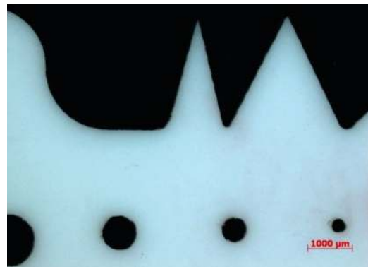
Figure 8: Complex contour cut with 10 mm/s with holes between 0.3 mm and 1.1 mm and sharp angles of 30° and 50°
