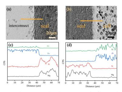
**Figure 6.** The SEM micrographs and EDS compositional profiles across the interface after 20 thermal cycles, under a compressive load of 0.3 MPa at 750 °C: seal/interconnect interface (**a**,**c**), seal/anode interface (**b**,**d**), exhibiting better interfacial compatibility.
