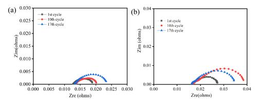
Figure 8. EIS of single cell stack at 750 °C at SOEC mode (a) and SOFC mode (b) under various.
