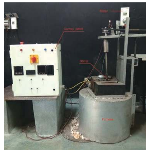
Fig. 5: Stir casting setup for fabricating Al7075 based hybrid composites
