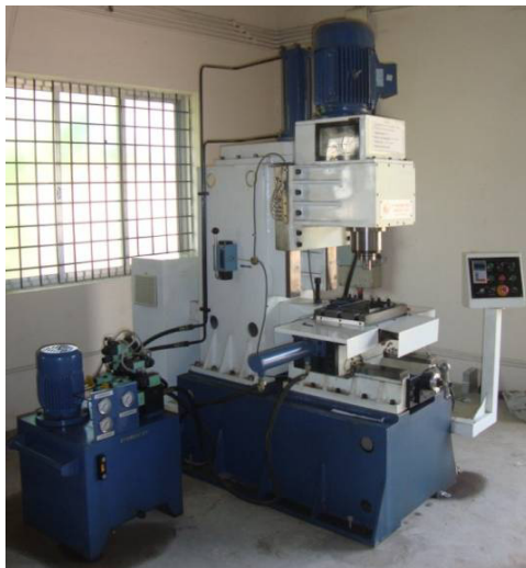
Fig. 2. Photographic view of FSW machine
