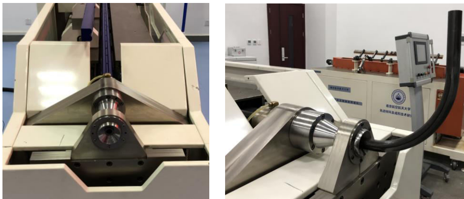
Fig. 8 Three-axial free bending forming equipment
