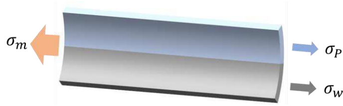
Fig. 7 Stress distribution of mixed uniaxial tensile specimen
