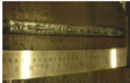
Figure 4. Photograph of chicken marks reported for weld of flux-cored arc welding.
