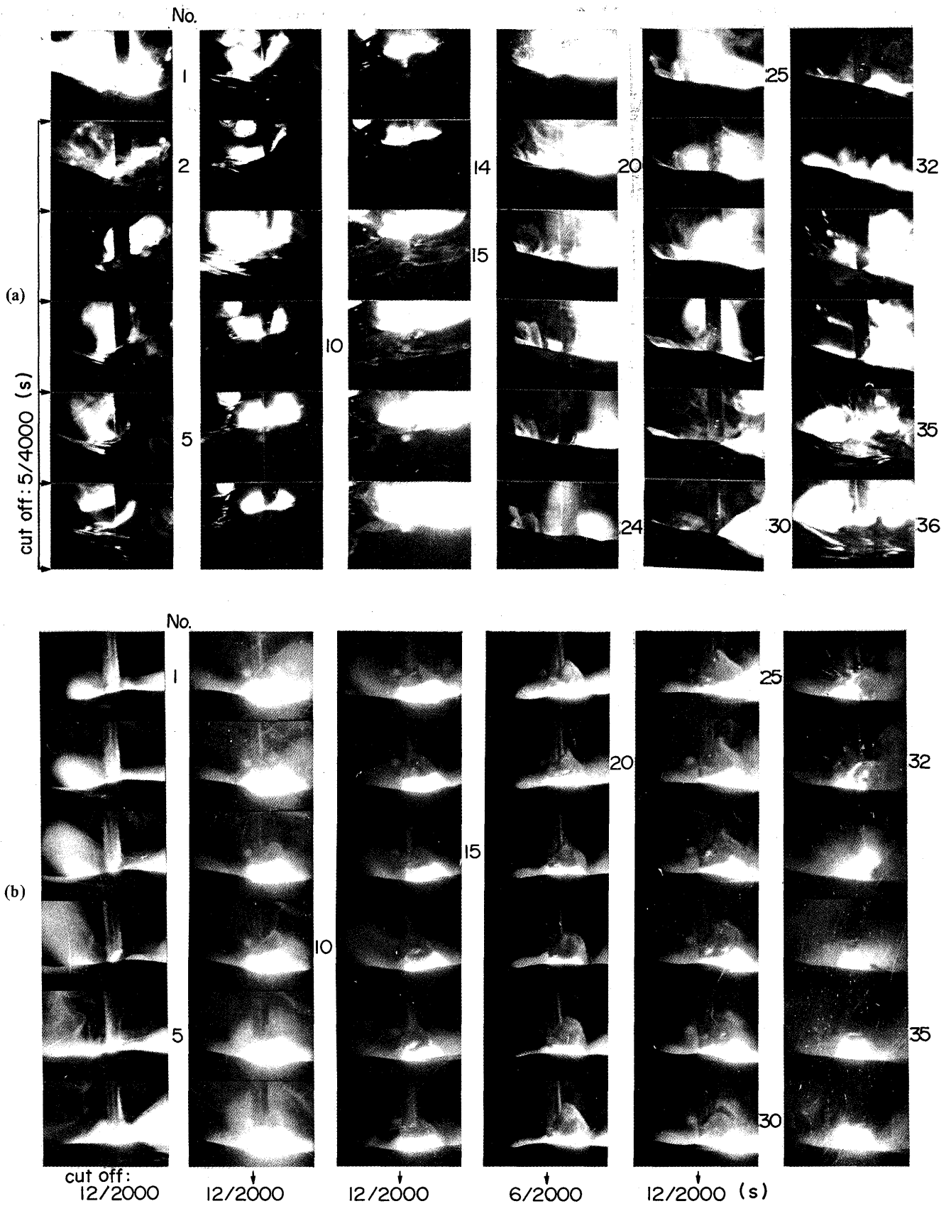
Fig. 5 High-speed motion photographs of molten metal. -(a): 400A, 32V (4000 frames/s), -(b): 400A, 32V frames/s, -(b): 400A, 38V (2000 frames/s)
