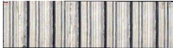
Fig. 2 Surface texture of a sample turned with the T2 tool point in real colour
