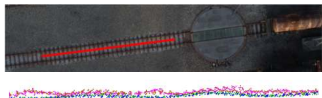
Figure 5. Presentation of the height profiles of the different point clouds in the track axis - profile position in the photo (top), point cloud profiles (bottom): P4D JPG80 (pink), P4D TIF (brown), PS JPG80 (green) and PS TIF (blue)
