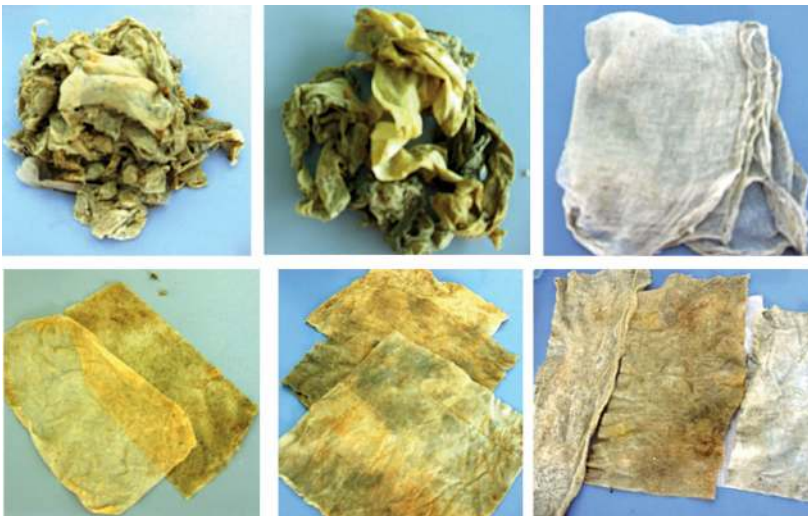
Fig. 11. Example constituents of scum layer in pumping station (based on one random sample), from top left to bottom right: paper lumps (paper), incontinence articles (composite materials), gauze (composite materials), wet wipes (different types, category nonwovens)
