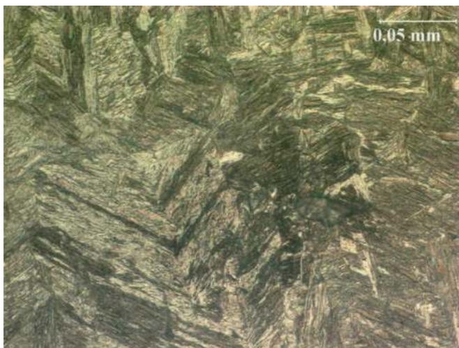
Fig. 14. Microstructure of DP600 weld: weld nugget, etched with 5-% nital, light microscope
