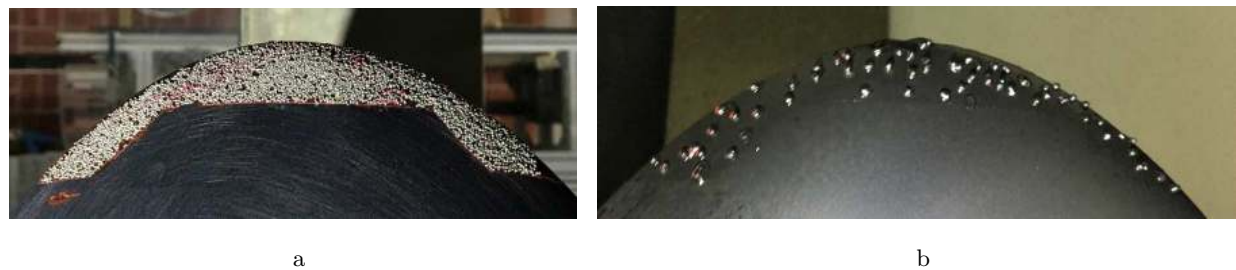
Fig. 5: Distributions of sand grains on the foil suction side, tip zoomed view. (a) Uniform distributions, (b) Sparse distributions.
