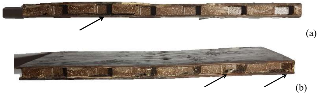
Figure 18. Failure analysis for rectangular (a) and hexagon panels (b).
