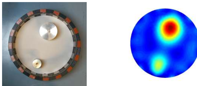
FIGURE 4. Left: An EIT measurement configuration for imaging objects in a tank. The electrodes used for measurements are at the boundary of the tank, which is filled with a conductive liquid. Right: A reconstruction of the conductivity inside the tank obtained using boundary measurements. [Jari Kaipio, Univ. of Kuopio, Finland; by permission.]
