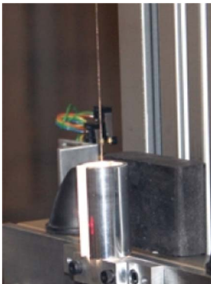
FIG. 8. (Color) Photograph of a ribbon being pulled. The heating zone and stock material are enclosed in a steel heat shield to minimize heat loss from the edges.
