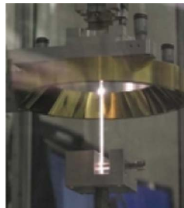
FIG. 6. (Color) The 3 mm diameter cylindrical fused silica stock being heated by the CO 2 laser as the fiber is pulled.
