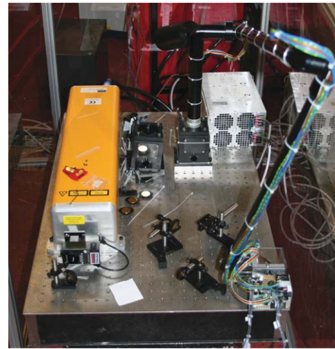
FIG. 9. (Color) The welding system consists of a CO 2 laser delivered through an articulated arm, ZnSe output telescope, and a pair of mirror galvanometers.
