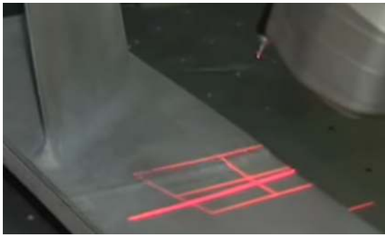
FIG. 4. Articulating arm laser line scanning of a turbine blade. (Reprinted from source: Martin Dury, NPL's National Freeform Centre.)
