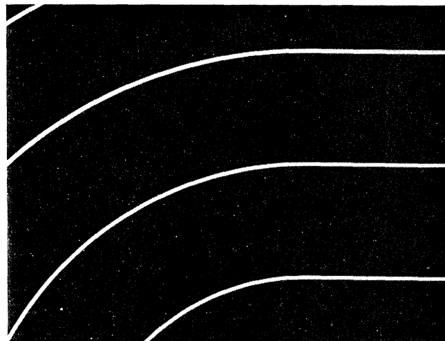
Fig. 7. Scribed metal photomask of optical guide pattern. Guide width is 10 \mu\text{m} .
