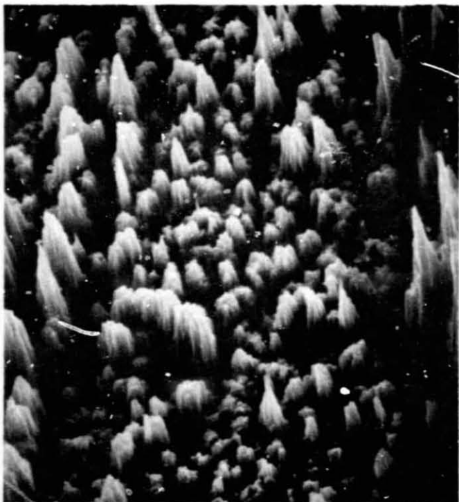
(a) PTFE SPUTTER ETCHED 0.5 HOUR BY 750 eV ARGON IONS AT 0.6 mA/cm 2 .
