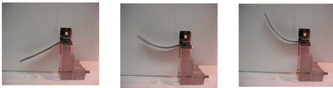
Figure 1. Successive photographs of an IPMC strip that shows very large deformation (up to 4 cm) in the presence of low voltage. Note that \Delta t = 0.5 s, 2 V applied. The sample is 1 cm wide, 4 cm long and 0.2 mm thick.
