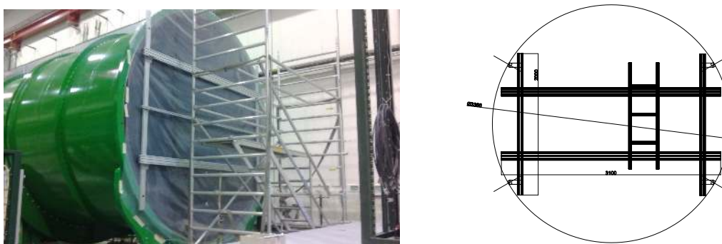
Figure 19. Left: the 2014 laser alignment support structure (at the upstream end of the RICH vessel). Right: the 2016 laser alignment support structure (inside the RICH vessel).
