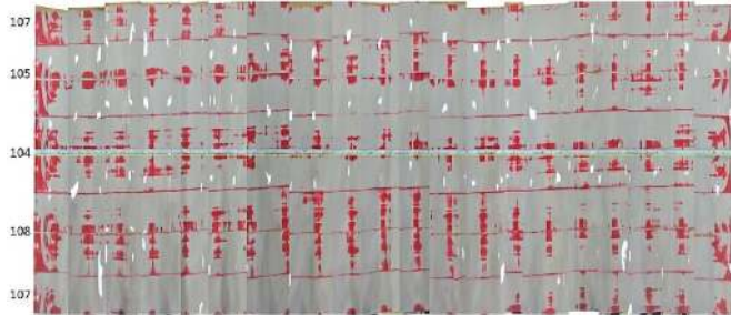
Figure 6. The FUJI film after the coil pack test assembly of MQXFBP1. The numbers on left hand side are the coil numbers. The pole of the coils are at the vertical positions of the numbers.
