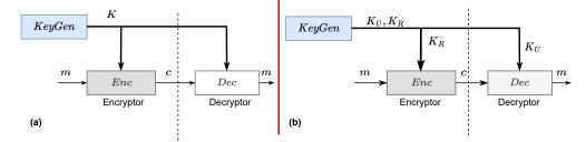
**Figure 4.** (a) A symmetric encryption scheme uses a single key, *K* for the encryption of a message, *m* and decryption of the encrypted message (cipher), *c*. (b) An asymmetric encryption scheme uses two different keys,  $K_U$  and  $K_R$ , for encryption and decryption.
