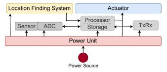
**Figure 2.** Major internal components of a sensor or an actuator. The component ADC stands for analog-to-digital converter, which converts an analog signal to a digital signal and vice-versa. TxRx stands for transceiver, which transmits and receives data from processor storage.
