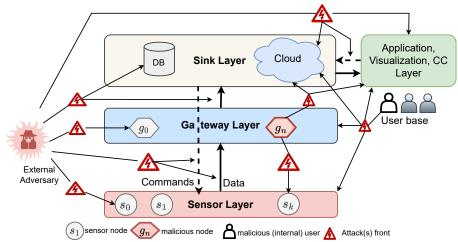
**Figure 5.** The threat model shows the components of the general IoT architecture and their interactions. Overall, the components and channels in an IoT form an attack surface. Three types of potential threat actors, viz., (i) external adversary, (ii) internal compromised (malicious) gateway device  $g_n$  in the gateway layer, and (iii) regular malicious (internal) user.
