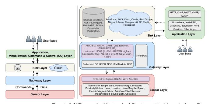
**Figure 1.** (Left) The general architecture of an IoT system consists of four major layers. The user commands and data from sensors become exchanged through the gateway layer. (**Right**) Popular instances of devices, protocols, or services in each layer of an IoT network. Discussion of the protocols and services is out of the scope of this article.
