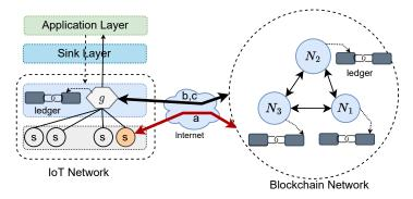
Figure 6. IoT and blockchain network integration models.
