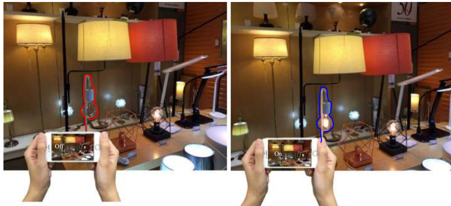
Fig. 8 AR interaction example of in situ/remote operation of the IoT lamp: the AR client provides an easy and intuitive way to turn on or off the lamp without having to control with the actual button or call the front desk for help (e.g., the red lamp in the left picture: the light is off, the same blue same lamp in the right picture: the light is on)
