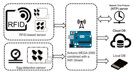
Figure 16. Block diagram of IoT platform for poultry-laying performance and behavior monitoring [70].
