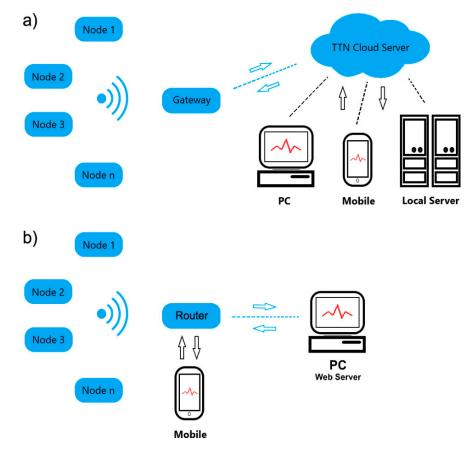
**Figure 12.** Sensor network operation scheme: (**a**) long range (LoRa) via The Things Network (TTN) cloud server [48], industrial scale or PaaS, (**b**) individual homestead, small-scale short-range.
