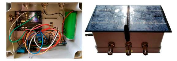
**Figure 10.** AMS: Arduino microcontroller with electronic components (**left**) and layout of ports and solar panels (**right**). Reproduced with permission from [37], Singidunum University.
