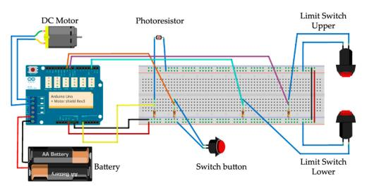
Figure 17. Arduino-based smart chicken coop door, DIY project [72].
