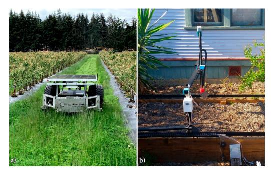
**Figure 15.** Autonomous machinery: (**a**) Directed Land Care Robot. Reproduced with permission from [59], 2020 Directed Machines; (**b**) FarmBot Genesis, photo by FarmBot, distributed under CC BY 4.0 license [63].
