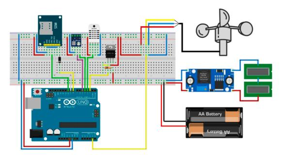
Figure 11. Arduino AMS based on the project described in [37], breadboard scheme.
