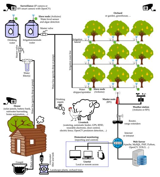
Figure 7. Integrated IoT based intelligent homestead automation system, high level overview.
