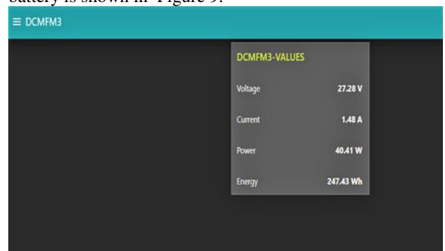
FIGURE 10. The display of battery parameters for 1 kW system
