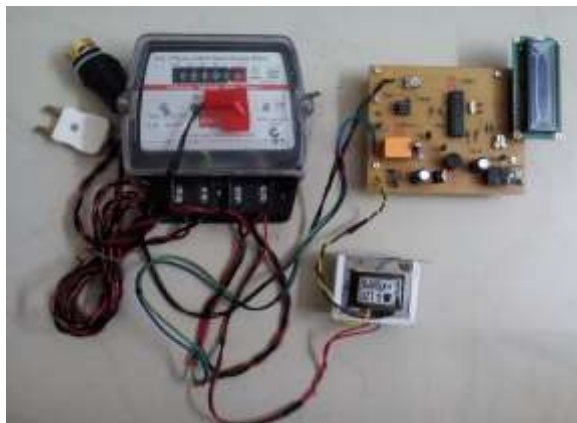
Fig. 5: Energy meter monitoring setup.
