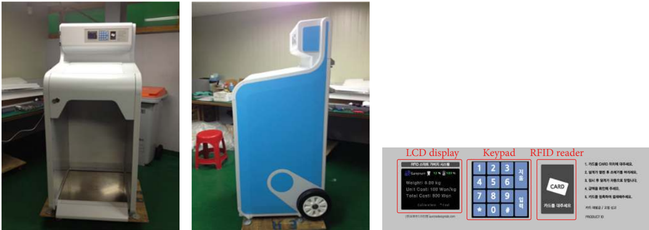
(a) Smart garbage bin (b) LCD display, keypad, and RFID reader
