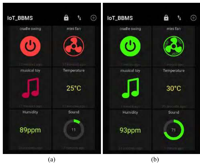
FIGURE 22. Sensor and actuator status: (a) OFF State; (b) ON State.
