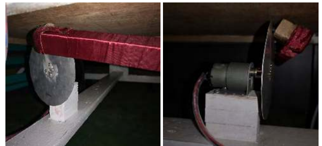
FIGURE 9. Rotating mechanism of the baby cradle.
